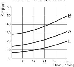
Note: Values measured on valve alone (no cavity) with an oil viscosity of 46 cSt at 50  $^{\circ}\text{C}.$  Pressure drop may change depending on fluid viscosity and temperature
