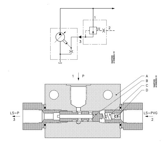
LS-PVG: Connection to LS-port, PVG LS-P: Connection to LS-port, pump Tallene 1, 2 og 3 are stamed into the valve
