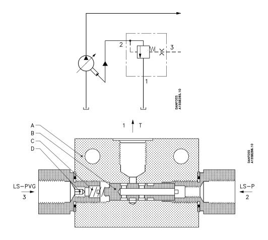
LS-PVG: Connection to LS-port, PVG LS-P: Connection to LS-port, pump Tallene 1, 2 og 3 are stamed into the val
