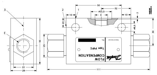
The numbers 1, 2, and 3 are stamped into the valve housing. E: G 1/4; 12 mm deep
