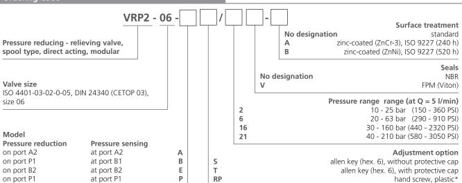
\*For pressure ranges 16 and 21 is possible to adjust reduced pressure only in circuit without pressure
