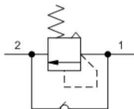
Atmospherically referenced, direct-acting sequence valves with reverse-flow check will supply a secondary circuit with flow once the pressure at the inlet (port 1) has exceeded the valve setting. Additionally, these valves incorporate an integral check valve to provide reverse flow from port 2 (sequence) to port 1 (inlet). The pressure setting of this sequence valve controls the pressure at port 1 relative to the atmospheric vent.
