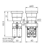
Weight 120 g Operating force 32 N Emergency - Rotate to unlock
