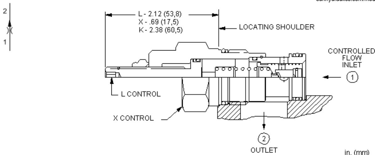
Fixed-orifice, pressure-compensated flow controls provide precise flow regulation for meter-in or meter-out applications where there may be wide pressure fluctuations. The flow setting is specified by the user and is set at the factory.
