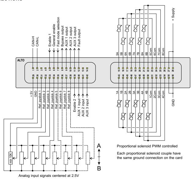
Joysticks can be supplied by an external stabilized supply, but the negative must be common with the STU card.
