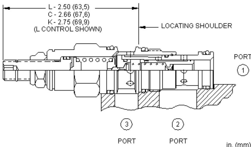
Pilot-operated, 3-way directional cartridges (1 blocked, 2 to 3 open) are switching devices typically used in moderate flow circuits. They can be used by themselves or to actuate larger pilot-operated directional cartridges or logic cartridges. The valve shifts when the pressure differential between port 1 and port 3 exceeds the setting.
