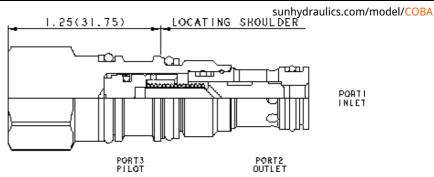
This valve is a spring biased closed, pilot-to-close check cartridge that has a 3:1 pilot ratio. The valve allows flow from port 1 to port 2 and blocks reverse flow. Pressure at the pilot port opposes pressure at port 1 at a ratio of 3:1. This valve is most often used in regeneration circuits.
