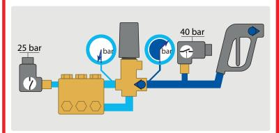
During the bypass phase water circulates in the pump without pressure.
