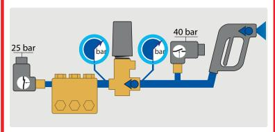
Reaching 25 bar the pressure switch (25 bar) changes the operating condition and secures the operation of the cleaner while pressure switch (40 bar) is deactivated.
