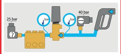
Contact of pressure switch (40 bar) is activated and by this way the cleaner can be started.
