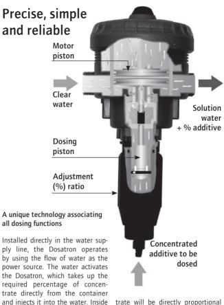
trate will be directly proportional to the volume of water entering the Dosatron, regardless of variations in flow or pressure, which may occur in the main line.
