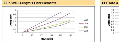
EFP Size 3 Length 1 Filter Elements with reverse flow valve
