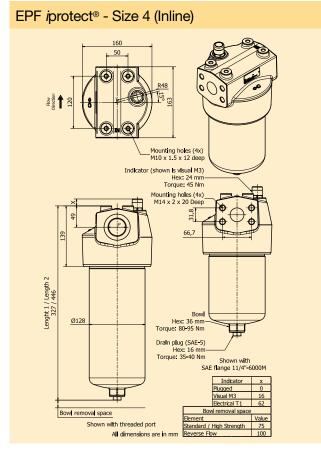
162 Hex 24 mm, Torque 45 km, Vent plus (SE-4) Hex 15 mm, Torque 35-40 km,
