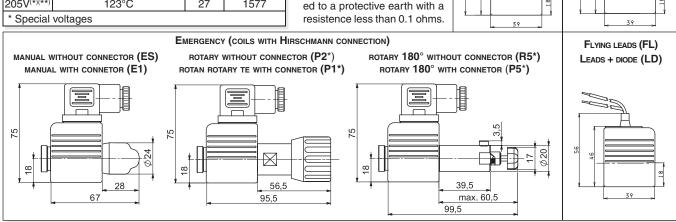
(\*) Emergency tightening torque max. 6÷9 Nm / 0.6 ÷ 0.9 Kgm with CH n. 22
