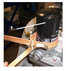
Replace the oil filter cartridge after the first 500 hours of use then every 2500 hours and in any event each time the oil is changed.
