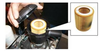
Remove the upper plastic shroud to gain access to inside the compressor.
