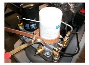
Replace the oil separator filter cartridge after the first 500 hours of use then every 2500 hours and in any event each time the oil is changed.
